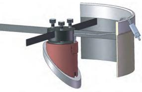
This illustration shows the heater installed after it has been wrapped around the cental stalk.
