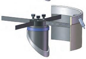
This illustration shows the neoprene heat insulator installed over the heater with the elastic band holding it in place.
