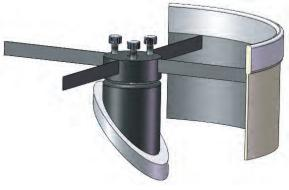
This illustration shown here is a cut-away showing a typical Newtonian secondary mirror holder that is used in many of today's Newtonaian and Dobsonian telescopes.
