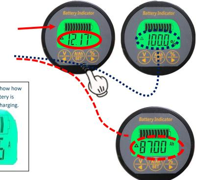
To switch between data-points, press the applicable button (V, A/Ah, %)
