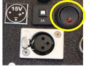
A toggle-switch turns ON output power. Turn OFF when not needed as it will deplete your battery if left ON
