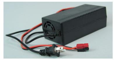
2) If the Power Pack was used in extreme temperature (hot or cold), allow the temperature to normalize before attempting to recharge. The internal "BMS" will only allow incoming charge current to pass when the battery internal temperature is within charging temperature range of 0°C ~55°C (32°F~131°F)
