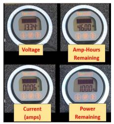
Because a LifePo4 battery has such a "flat" voltage curve, we can't use voltage as an indicator of remaining available power. The Battery Monitor uses a "shunt" and continuously meters incoming and outgoing power.
