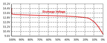
A major advantage of Lithium Iron Phosphate is relatively "flat" voltage curve. Beware that excessively large loads will cause voltage to drop below the normal voltage curve.
