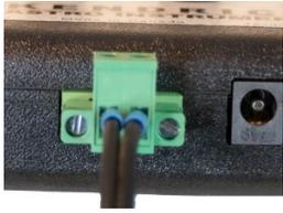
The standard power cord uses a cigarette lighter plug at one end and a special “terminal block” plug at the other. The device plug has 2 screws that secure it to the controller. A jewellers (small) slotted screw driver works well.
